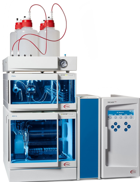
Figure 4. Recommended instrument configuration for this application: the ALEXYS Carbohydrate Analyzer. The system consists of an ET210 Eluent tray for nitrogen blanketing, a P6.1L quaternary LPG pump capable of running gradient program, an AS6.1L autosampler, a CT2.1 column thermostat, and a DECADE Elite electrochemical detector. The ALEXYS Carbohydrate Analyzer can be fully controlled by different Chromatography Data System (CDS) software, namely DataApex™ Clarity™ CDS (version 8.3 and up) or Thermo Scientific™ Chromeleon™ CDS (version 7.2 SR5 and up).
